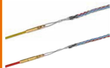
CALZE TIRAFILI Cable pulling grip SA017801 ø mm 6-9 L. mm 200 Brake load Kg 220 SA017802 ø mm 9-12 L. mm 250 Brake load Kg 440
